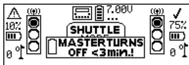
Master critical battery
